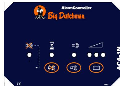
The ACA-1N is an alarm device with a single alarm input, allowing connection of signallers like a horn, a flashing light, HBA and a telephone selector contact. Setting an alarm delay and suppression time is possible as well as continuous monitoring of charge and discharge current. Every 24 hours the battery capacity is checked and an alarm is released at capacity drop below a set value.
